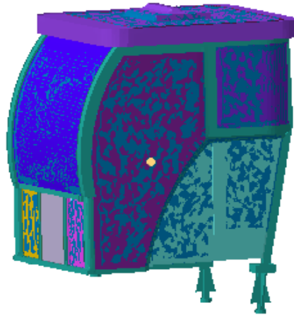
Figure 1. Cab acoustic-solid coupling model
